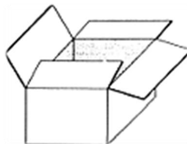
Regular Slotted Container RSC
